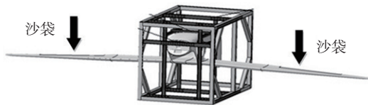
图7 整机静力试验 Fig.7 Static test of aircraft
